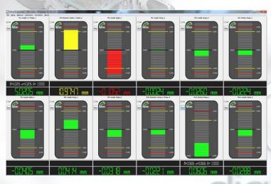
General **Cyberus®** application software allows you to define measuring task profiles at your choice. For example defining a shaft measuring task either between centers or in vee prisms is easy. The built in math parser allows you to define mathematical operations needed for most measuring tasks.
