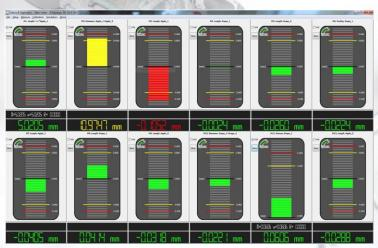
General **Cyberus® Compact** application software allows you to define measuring task profiles at your choice. For example defining a shaft measuring task either between centers or in vee prisms is easy. The built in math parser allows you to define mathematical operations needed for most measuring tasks.
